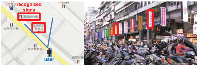
Fig. 8. The information on the GPS map and the corresponding recognized shop signs in the video frame
